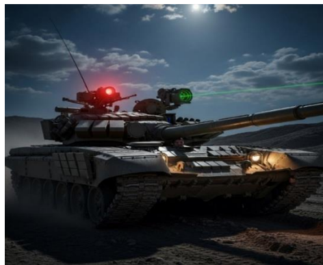
Figure 32: A T-90 equipped with "Shtora-1" Electro-Optical/Infrared system
