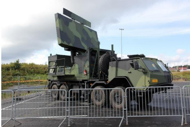
Figure 28: A Finnish Ground Master 400. It is a mobile long range radar system which can detect tactical aircrafts, UAVs and cruise missiles.
